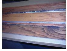
On the left is a manufacturing issue. The boards were treated with a darkening agent to simulate a distressed look. Uneven application resulted in heavy staining and blotches. The owner rightly refused the shipment of flooring.
