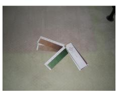
On the left is a carpet manufacturing issue – fume fading. The carpet started out tan and gradually turned light green. A hope chest was moved revealing the original color. The item in the middle of the picture is a 'Gray Scale' kit.
