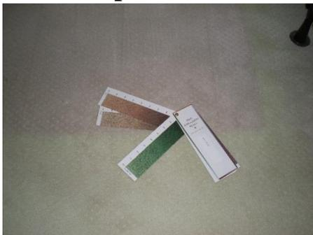
On the left is a carpet manufacturing issue – fume fading. The carpet started out tan and gradually turned light green. A hope chest was moved revealing the original color. The item in the middle of the picture is a ‘Gray Scale’ kit which allows me to tell the manufacturer exactly the magnitude of color change.
