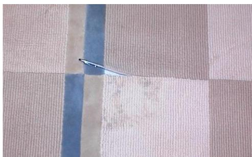
On the left we have a ‘Specification’ issue. They used the incorrect face yarns. This hand cut wool carpet was installed on a boat. Wool is prone to mold damage when exposed to high humidity situations, such as an enclosed boat. Also the glue used on the backings was inappropriate as it failed due to the high moisture levels.
