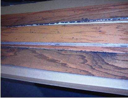
On the left is a manufacturing issue. The boards were treated with a darkening agent to simulate a distressed look. Uneven application resulted in heavy staining and blotches. The owner rightly refused the shipment of flooring.
